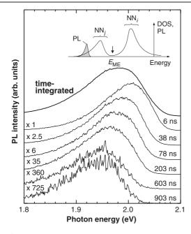
**Figure 1.** Photoluminescence spectra of a GaP<sub>0.979</sub>N<sub>0.021</sub> sample taken at different times after the excitation pulse and a time-integrated spectrum (integrated over the first 10 ms after the laser pulse). The inset illustrates schematically the density of states (DOS) due to nitrogen clusters, the position of the mobility edge  $E_{\text{ME}}$ , and the PL signal.
