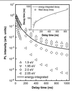
**Figure 2.** Decay of the PL intensity of selected photon energies (symbols). The solid line shows the decay of the energy-integrated PL intensity. The inset illustrates a transient evolution of the PL decay time determined from the energy-integrated PL intensity (solid lines) and that determined from the theoretical fit to the experimental data in figure 3 (open symbols).
